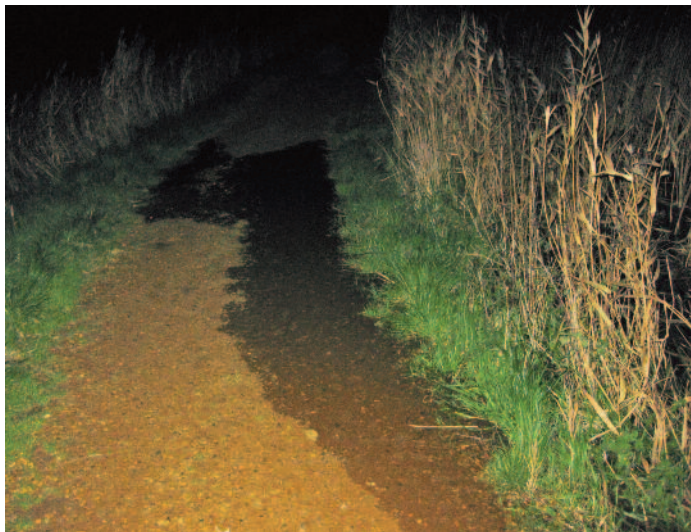
Overtopping starting at 12.41am about 150m East from Snape Bridge. This, taken with the gauge readings should give an indication of total overtopping levels through the surge. Approx grid ref TM 3931 57632.
